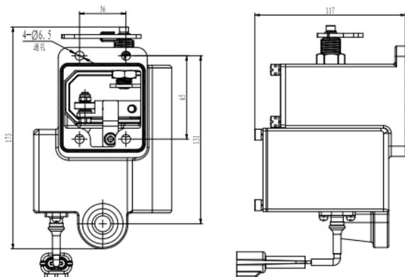
Figure 2.2.5 The outline and installing size of the A08A-W electromagnetic actuator
