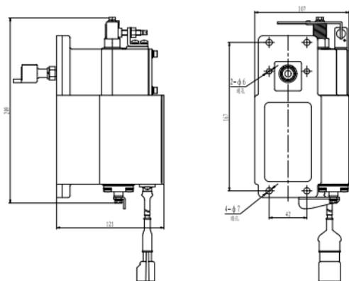
Figure 2.2.6 The outline and installing size of the A3A-W electromagnetic actuator
