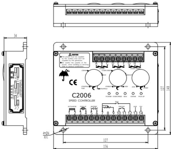
Figure 2.1 The outline overall and installing dimension of controller C2006
