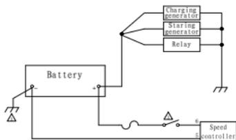
☑ The correct wiring diagram
