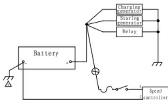
☒ The wrong wiring diagram
