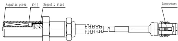
**Figure 2.3** Speed sensor structure diagram
