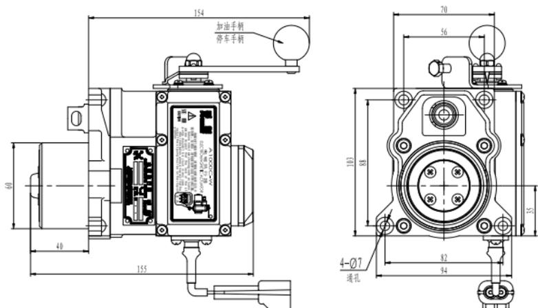
Figure 2.2.3 The outline and installing size of the A1000C-W-d1 electromagnetic actuator
