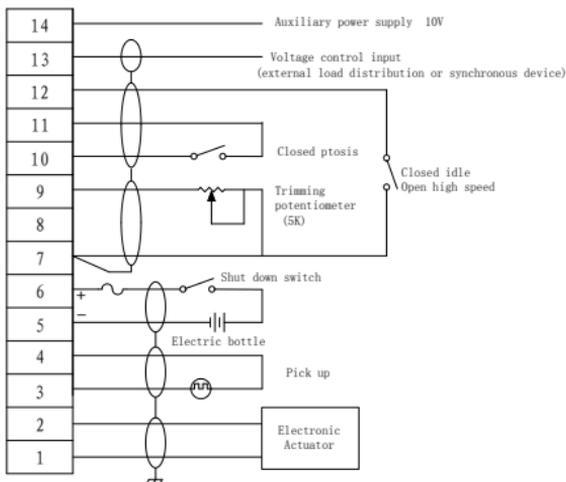
Figure 2.2 The wiring diagram of speed controller C2006
