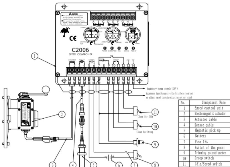
Figure 3.1 Connection diagram of the ESG2006 series electronic governor system
