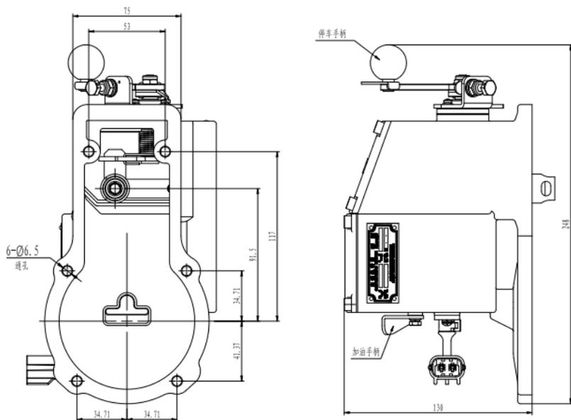
Figure 2.2.2 The outline and installing size of the A800C-W electromagnetic actuator
